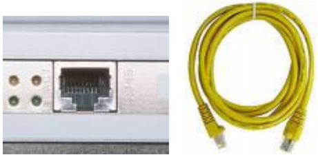
Figure 6. Ethernet port and cable
