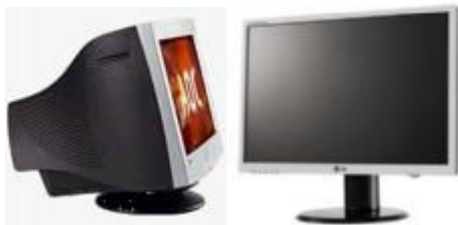
Figure 4. CRT Monitor on left, TFT on right.
