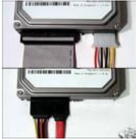
Figure 2. Top connector is IDE, bottom one is SATA-II
