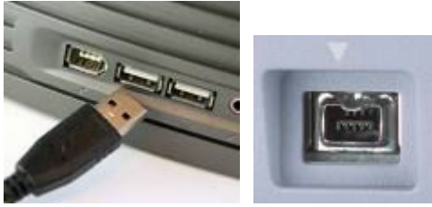
Figure 8. USB (left) and Firewire (right) ports
